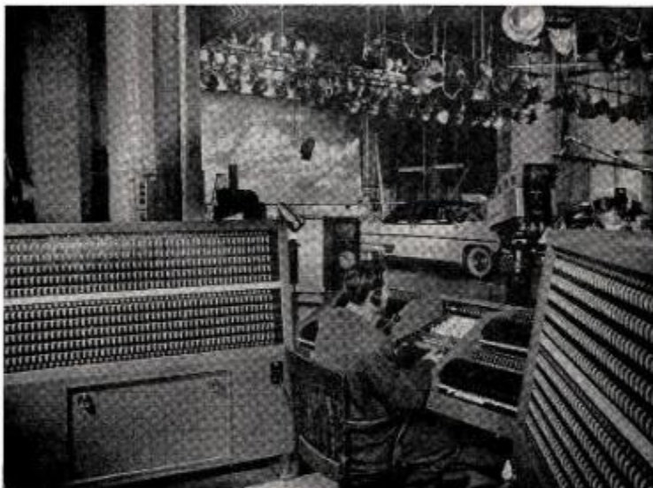
THIS ORGAN-LIKE CONSOLE will control the elaborate lighting for color tv productions at CBS-TV's New York Studio 72. The operator is seated at an Izenour board which pre-sets light cues and stores them in "memory boxes." The board controls 500 individual stage-lighting fixtures. The studio was inaugurated yesterday (Sunday).
