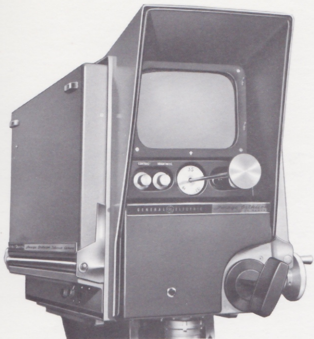
Rear view of I.O. camera. Shown are 8" viewfinder, center shaft zoom lens control, viewfinder controls, lens position indicator, lens selector handle, focusing knob.
