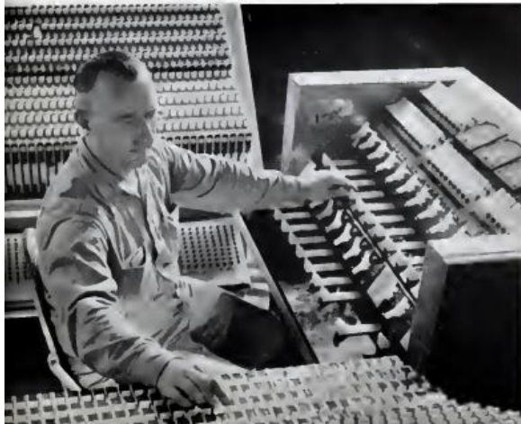
At the "Lumi-Tron" lighting board, 2,000 lighting controls are within reach of the technician.
