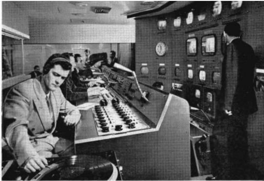
NBC Studio 5H at opening in December. Technicians man console while broadcast coordinator occupies glass-paneled booth at left, facing large monitor panel at right of picture.
