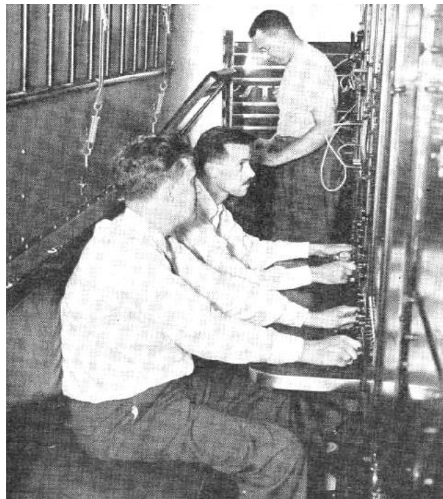
FIG. 44.—The television mobile unit. The upper unit is equivalent to a studio control room; the lower unit contains the radio transmitter used to relay the television signal to the Empire State Building for rebroadcast on the main transmitter.
