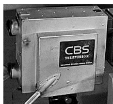
The Gray Telop, with four optical openings affording dual projection from any two channels. Note control panel, slide holders.
