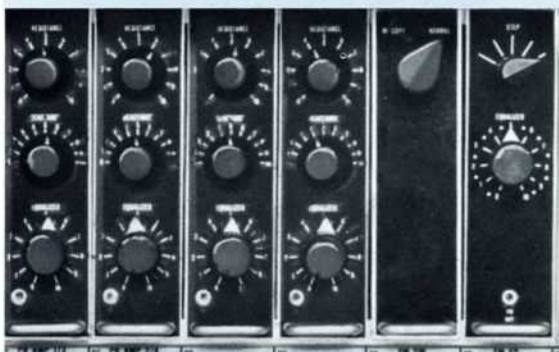
Ability to match the individual head responses is provided by the RESISTANCE, REACTANCE, and EQUALIZATION controls.
