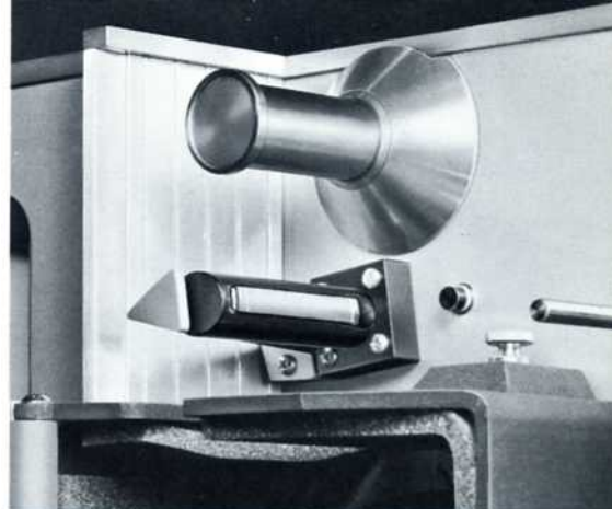
The use of a rear side erase head minimizes the possibility of scratching the oxide surface of the record tape.
