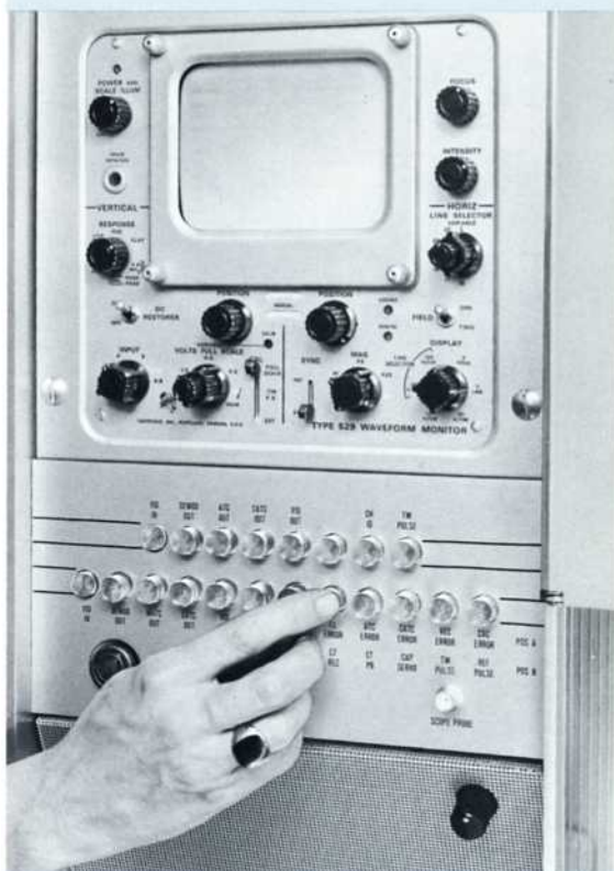
The wide range of built-in monitoring is further expanded through the use of an external scope probe. The probe can be used to view the waveforms at the module test points.
